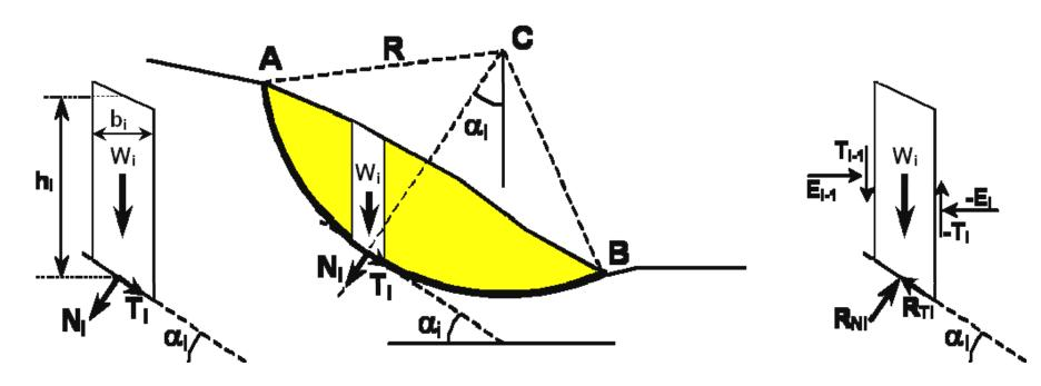
The resolution needs a way to distribute the contact normal force on the limit of the block
